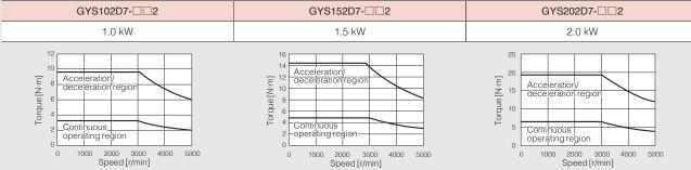
These characteristics indicate typical values of each servomotor combined with the corresponding RYT-7 type servo amplifier.
