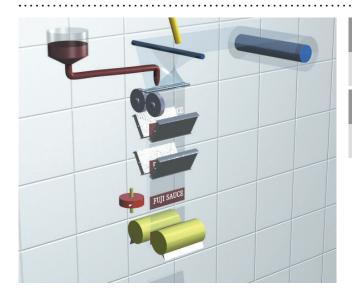
Solution 1 To eliminate defective workpieces by synchronizing the feed, seal, and cut axes
